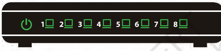
Figure 10.11: A network hub with 8 ports
